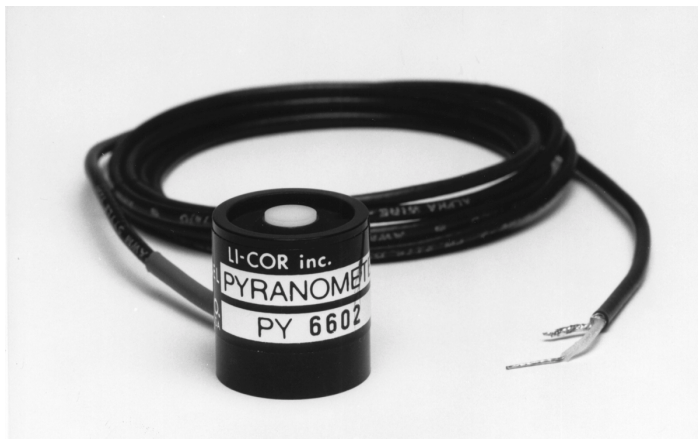
Figure 1. "SZ" type sensors have no connector and are terminated with only the bare wire leads of the coaxial cable.
