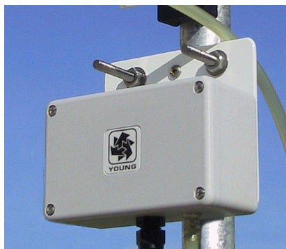
61202 Barometer mounted on mast.
